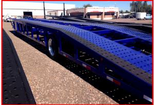
The Sun Country Trailers Air Ride/Air Brake 3 - Car Hauler is our original Road Tractor car carrier. With 53' of useable space it became popular for clients who haul high profile vehicles, such as vans or full size trucks. The Air Ride suspension helps provide a smoother ride as well as provide a dump valve to lower the suspension while loading and unloading.
